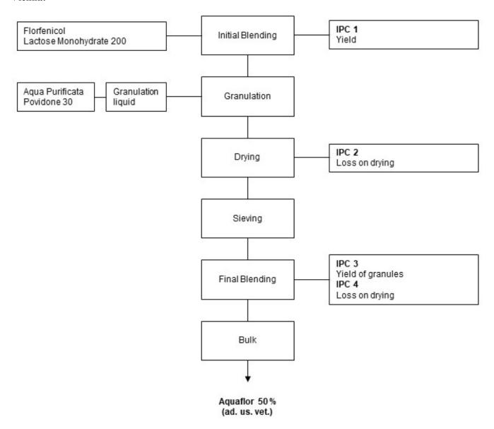
(b) Narrative summary of the fabrication process, including amounts of ingredients, equipment type, process parameters, in-process testing with acceptance criteria:
